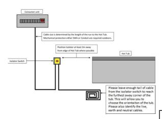
The rotary isolator switch should be at least 2 meters from the hot tub, and it must not be possible to access the switch from inside the tub. On the other end of the isolator the electrician should connect and coil up 4-5meters of Cable SY or SWA cable (or possibly more depending on
